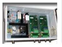
**ZUC I/O IP:** Communication card Input and Output under IP.
